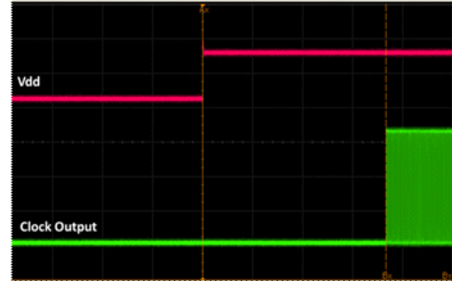
Figure 16. Startup Waveform vs. Vdd
