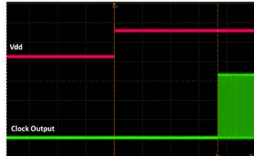
Figure 16. Startup Waveform vs. Vdd
